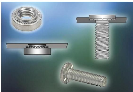
**Manufactured from hardened alloy steel, SHTM hard panel nuts and HFLHTM hard panel studs are designed for installation into especially hard sheet materials, such as high-strength steel. Photo courtesy PennEngineering**
