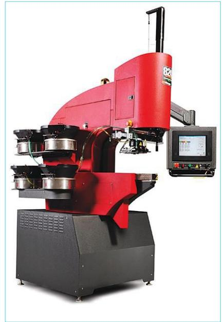
**SingleTouch Part Handling Technology enables a press to insert up to four different self-clinching fasteners in a single handling of a part.**
