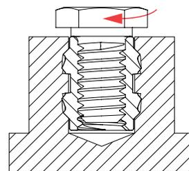
**Torque-out** is the torque required to turn the fastener in the parent material after installation without inducing clamp load on the fastener.
